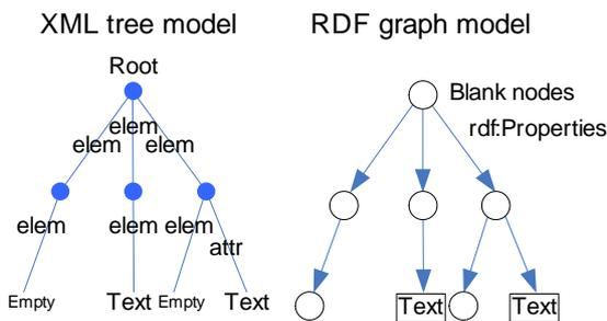
Figure 4. XML tree and resulting RDF graph models
